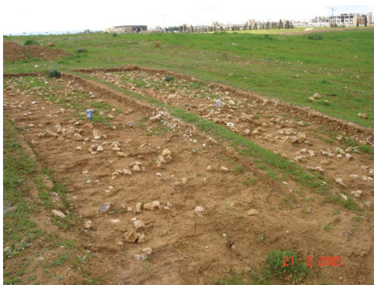
Figure 1. General view for the experimental plots; the 15% stone cover plot is shown in the right and the 5% stone cover plot is on the left.
